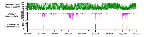
Fig. 3. Renewable generation (top), energy in storage (middle), and fossil generation (bottom) for the four-year study period in the 99.9% coverage case with GIV storage and 2030 technology costs. Scales are GW generated and GWh held in storage.
