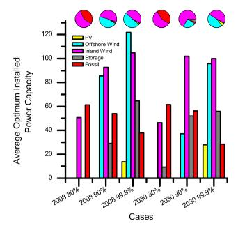
**Fig. 5.** Power capacity of generation and storage (bars) and source of energy used to meet load (pie charts) in all 18 RREEOM runs. Each cluster of bars (e.g. the 4 bars labeled "2008 90%") and pie chart above are an average of the three storage technologies.
